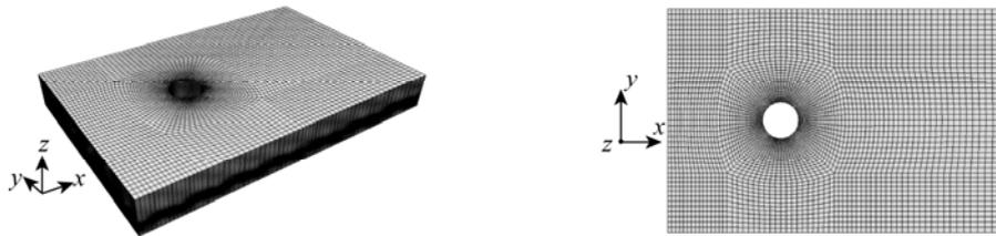
Fig. 6. Mesh of the computational domain.
